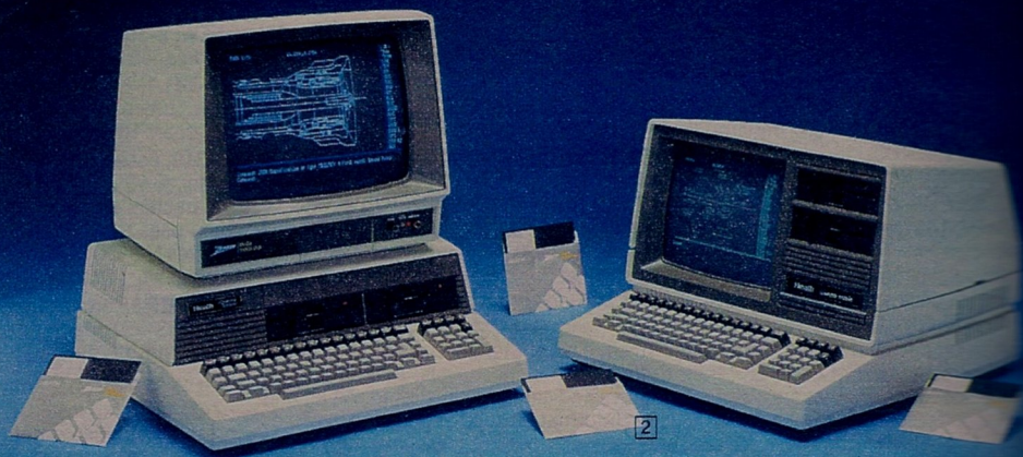
H-100 Low-Profile Computer with optional ZVM-135 and second floppy disk drive
