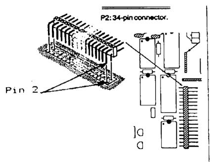
Figure 3. Pin 2 of the 34-Pin Connector
