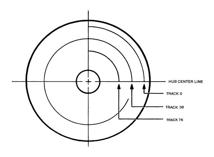
Figure 2-2 Hub Center Line and Track Locations
