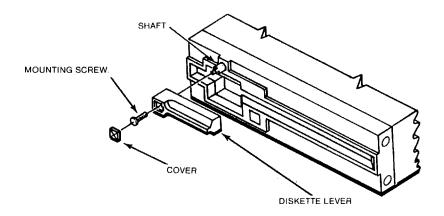
Figure 5-6 Diskette Lever Key Parts
