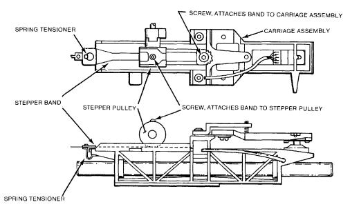
Figure 5-20 Stepper Band Key Parts
