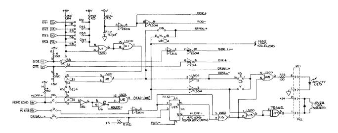
Figure 1-10 Radial Head Load Signal
