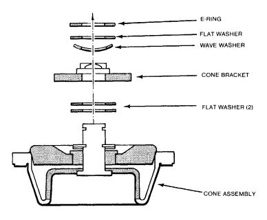
Figure 5-5 Cone Assembly Parts
