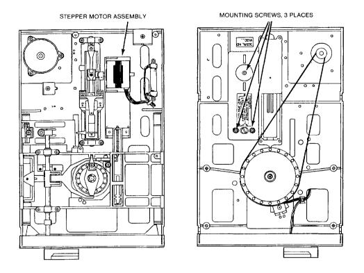
Figure 5-21 Stepper Band Additional Key Parts
