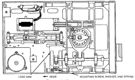
Figure 5-12 Load Arm Assembly Key Parts
