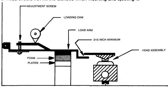
Figure 2-12 Load Arm Adjustment, Front View
