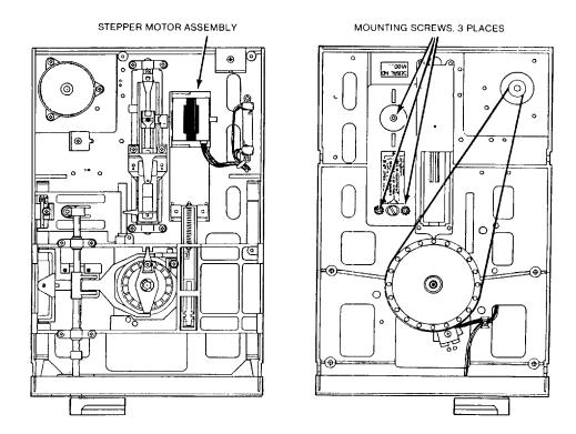
Figure 5-22 Stepper Motor Assembly Key Parts
