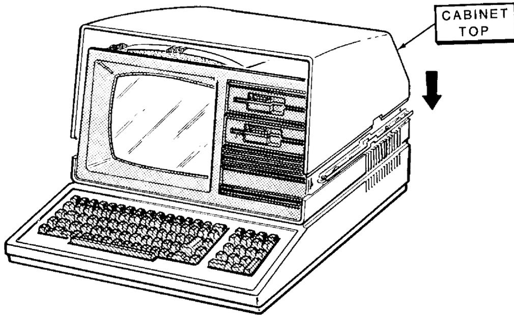
**Figure G-16: Replacing the Cabinet Top**
