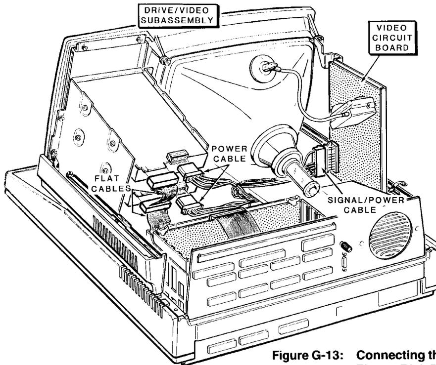
**Figure G-13: Connecting the Signal/Power and Floppy Disk Drive Cables**
