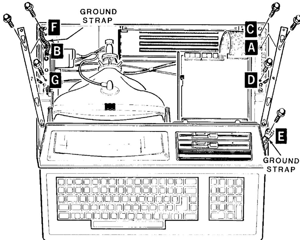
**Figure G-2: Unfastening the Drive/Video Subassembly**
