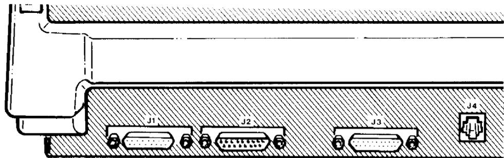
**Figure 1-4: Peripheral Connectors**
