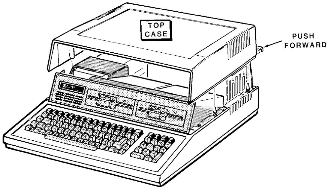
**Figure G-20: Replacing the Cabinet Top**
