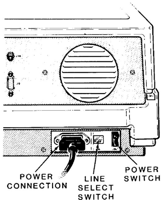
**Figure 1-5: Power Connectors and Controls**
