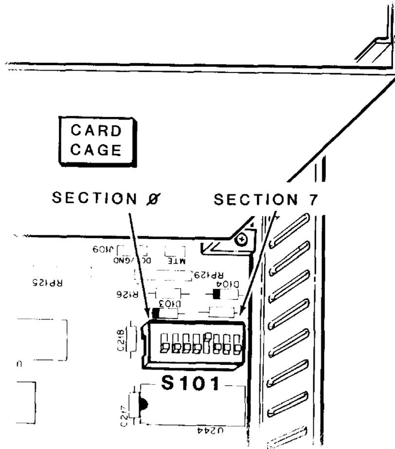
**Figure G-21: Switch S101 (Main Board)**
