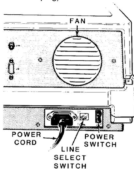
**Figure 1-6: Power Connections**
