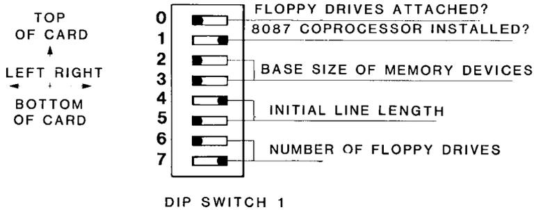
**Figure 4.2. DIP Switch SW1 Settings**
