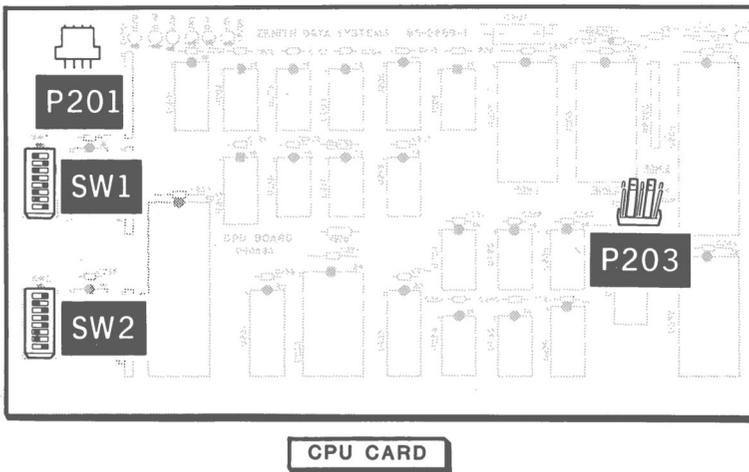
Figure 4.1. CPU Card Component Locations
