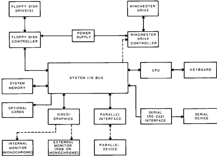
**Figure 3.1. System Block Diagram**
