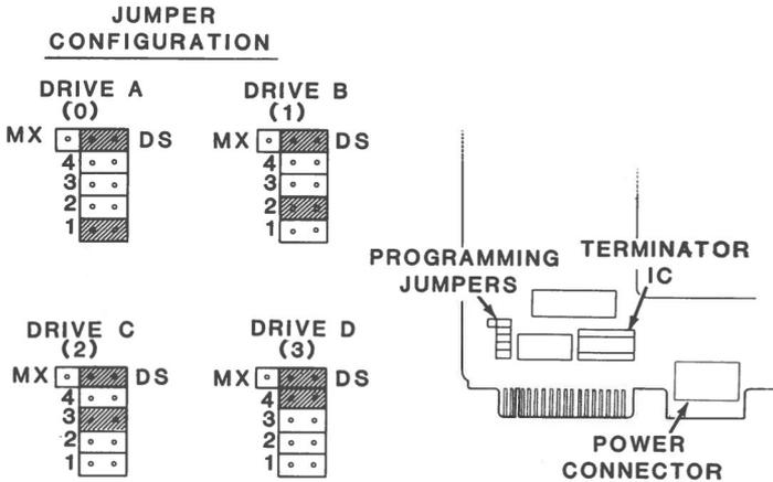
Figure 9.3. Shugart Floppy Disk Drive Configuration
