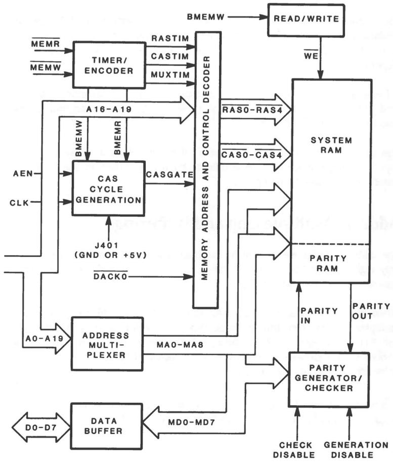
Figure 6.2. Memory Access Block Diagram
