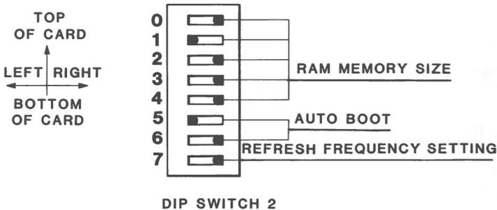
Figure 4.3. DIP Switch SW2 Settings
