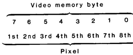
**Figure 7.6. High Resolution Mapping**
