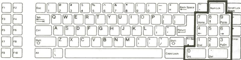
Figure 5.6. Keypad Special Keys
